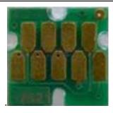
To determine the precise location of the terminals' contact portions, the following steps were taken: (1) using a marker, black ink was applied to the terminals and the terminal arrangement photographed; (2) the Representative '116 Ink Cartridge was installed in and removed from the printer; and (3) the terminal arrangement was photographed. The following photo shows the terminals after the application of black ink with a marker.
