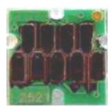
The step of installing and removing the cartridge from the printer, causes the printer's contact forming members (discussed at 18(a), *supra*) to leave scratch marks on the terminals thereby removing a portion of the black ink that was applied with the marker. The following photo shows the terminals after the cartridge was installed and removed from the printer.
