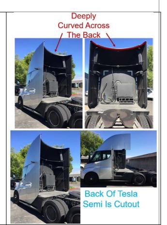
As the above comparison shows, the striking dissimilarity between the two fuselage designs is undeniable when viewed from the back and top—*i.e.*, the two views Nikola omitted from its FAC. These views confirm that there can be no infringement. First, the top view demonstrates that, in the patented design, the back edge of the top surface of the fuselage is a straight line. In stark contrast, the back edge of the top surface of the Tesla Semi is deeply curved rather than straight.
