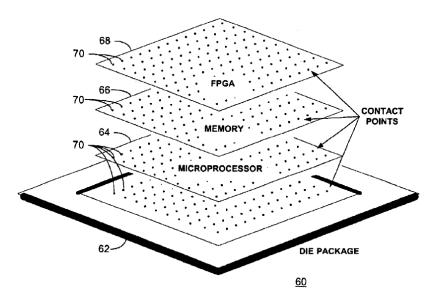
(*See* D.I. 1, Ex. 1-4 at 1) The Patent describes this figure as showing "processor module in accordance with the present invention comprising a hybrid device incorporating a number of <u>stacked</u> integrated circuit die elements." (*Id.*, Ex. 1, 3:29-32, Ex. 2, 4:3-6, Ex. 3, 4:5-8, Ex. 4, 3:25-28)
