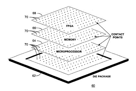
(*See* D.I. 1 at Ex. 1-4 at 1; figure description at D.I. 1 at Ex. 1, 3:29-32, Ex. 2, 4:3-6, Ex. 3, 4:5-8, Ex. 4, 3:25-28 ("[The figure] is a . . . view of a reconfigurable processor module in accordance with the present invention comprising a hybrid device incorporating a number of <u>stacked</u> integrated circuit die elements."))
